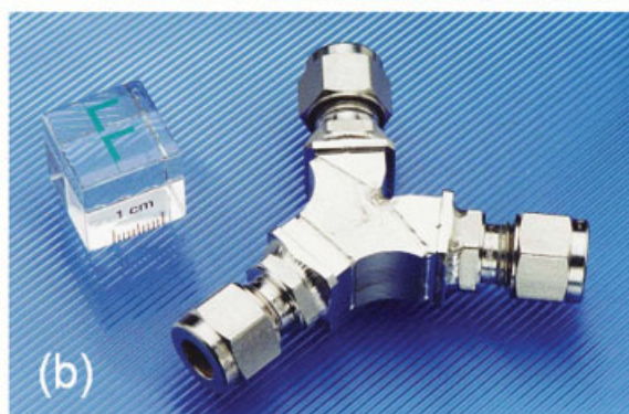
Figure 5. Construction principle (a) and photo (b) of parallel mixer (P-type mixer).
